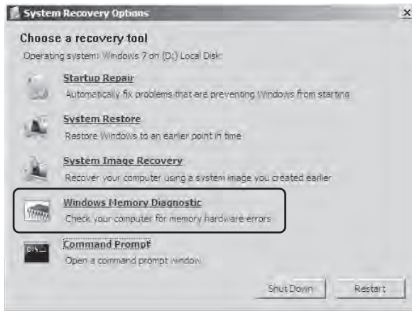
FIGURE 1-30 Selecting the Windows Memory Diagnostic recovery tool
